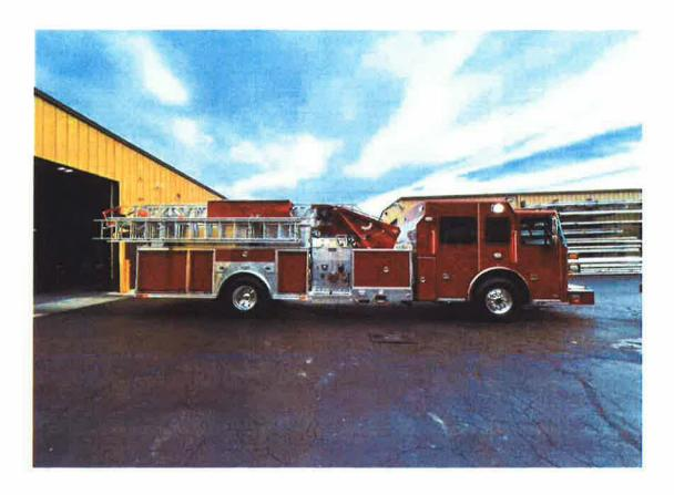
Chief Robinson shared the photo of the recommended next engine, called a "Quint". This is a Sutphen SL75 Quint-style truck. This vehicle models the current fire engines and includes a 75' aerial ladder (this is NOT a ladder truck). This additional resource would allow the Fire Department to reach the taller warehouses and hotels that have been built within the Township.
